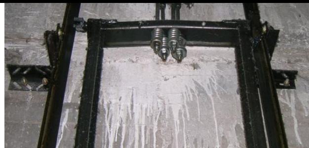
Counterweight frame bent
